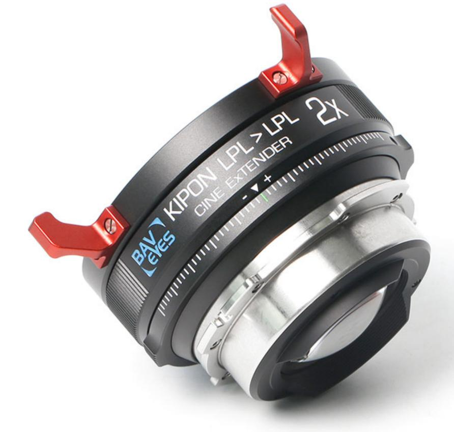
An integrated option to finely adjust the flange focal distance via rotary wheel (FFD Adjustment +/- 0.05mm), allows a quick fine tuning of the flange focal distance without the use of tools and shims. The adapter is pre-adjusted to 44.00mm flange focal length (LPL FFD) ex works.
